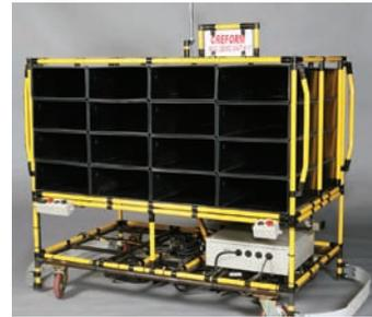
This compartmented vehicle has 32 spaces total for safely transporting sequenced assembly components, kitted materials or fragile, delicate components. The cart was created using the Creform system of pipe & joints and the addition of a Creform AGV drive unit power source converts it to an AGV.
