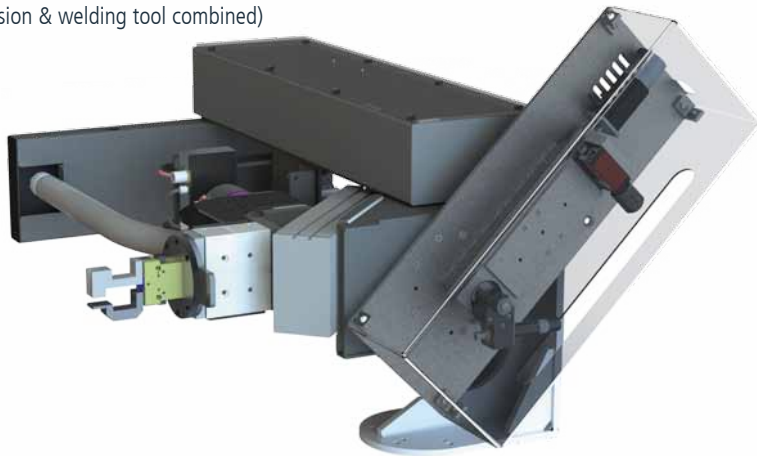
Robot end of arm tool (vision & welding tool combined)
