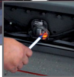
Logic modules are set in the field with the simple press of a button.
