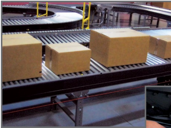
In non-contact accumulation, products accumulate but do not touch.
