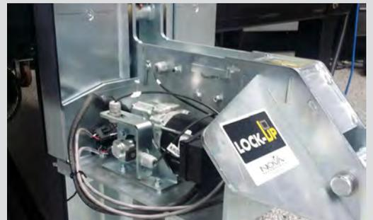
Sealed magnetic proximity sensors with direct drive gear motor
