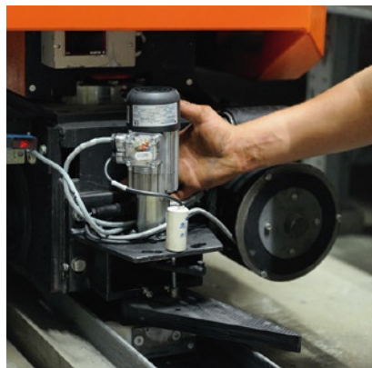
Current (2009) switching technology with redesigned rail-switching drive and rail switches. The new points are built to minimize wear and tear.
