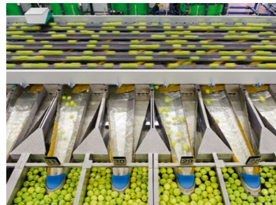
The new sorting system classifies up to 65 apples per second on the basis of a 3D model, which is assessed out of 60 pictures for each single apple.
