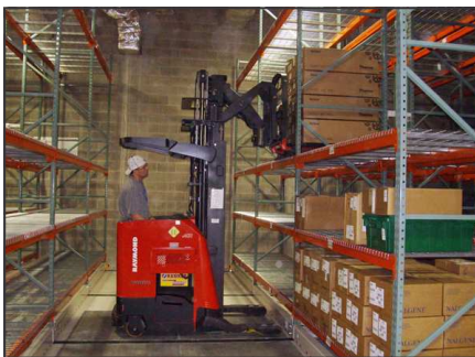
Reach truck accessing open rack area (left, top and bottom). Mobile rack in closed position (right).
