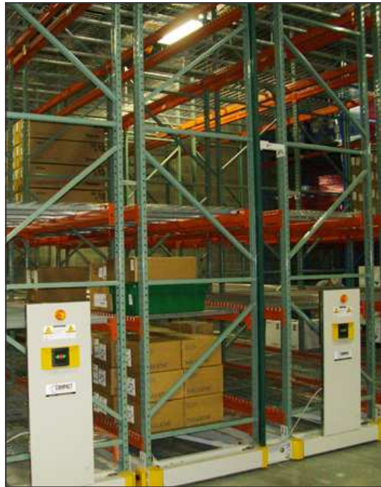
Reach truck accessing open rack area (left, top and bottom). Mobile rack in closed position (right).
