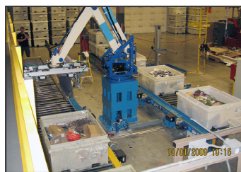
Fuji EC201 Robotic Palletizer
