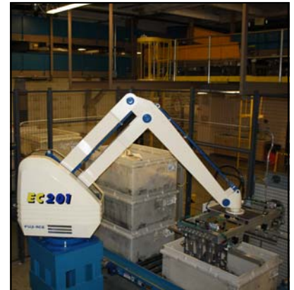
The Fuji EC-201 robot stacks and destacks totes filled with consumer products.
