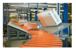
That is why Zalando has selected the deniway plate chain conveyor: both lines with an overall length of around 410 metres each require just two 2.2 kW drive units. So Zalando makes big savings on energy. And because the cardboard packaging is now easier to handle, it is possible to optimize resources further. When Zalando grows, then thanks to its modular design, deniway simply grows with it.
