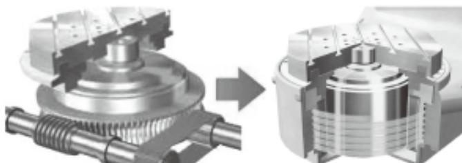
Fig.5 Worm Gear System and Direct Drive System
